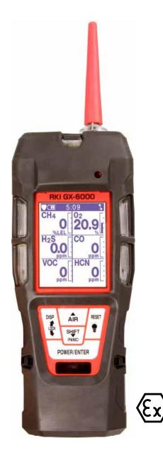
**GX-6000**Portable multi gas detector
